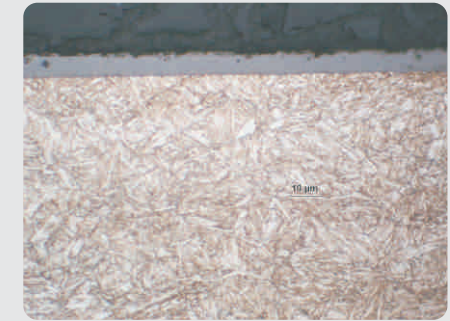
Nital: iron oxide Fe 3 O 4 , thickness 9mm and tempered martensite
